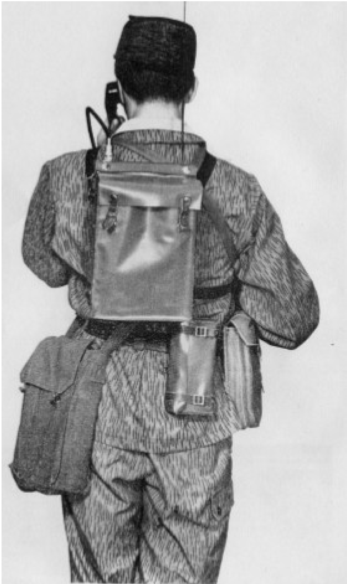
Figure 8: The radio in a bag worn on the back – rear view – spare battery bag vertical
