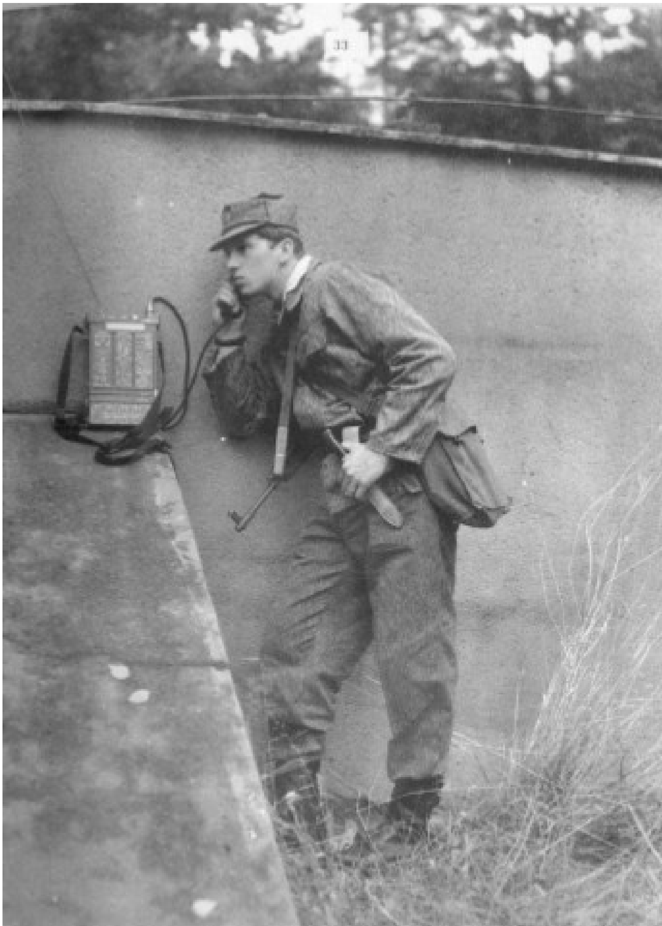
Figure 17: Use of the antenna to use the cover provided by a wall
